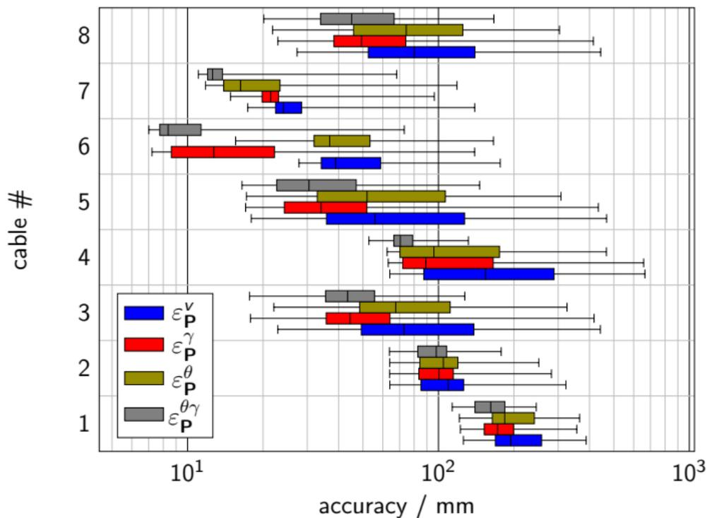
Figure: Accuracy of the models for each cable.
