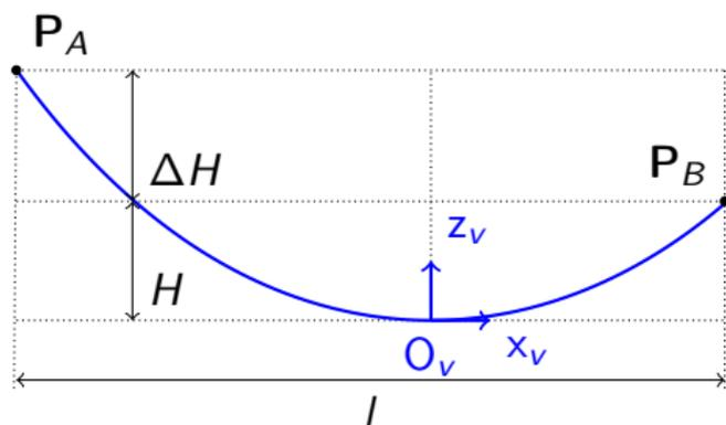
Figure: Catenary of length  $L$  hanging between  $\mathbf{P}_A$  and  $\mathbf{P}_B$ .
