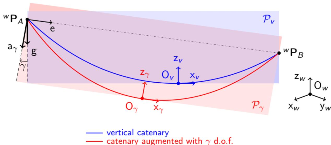
Figure: Standard and  $\gamma$ -augmented catenary [Drupt et al., 2022] of length  $L$  hanging between  ${}^w\mathbf{P}_A$  and  ${}^w\mathbf{P}_B$  in their respective planes.
