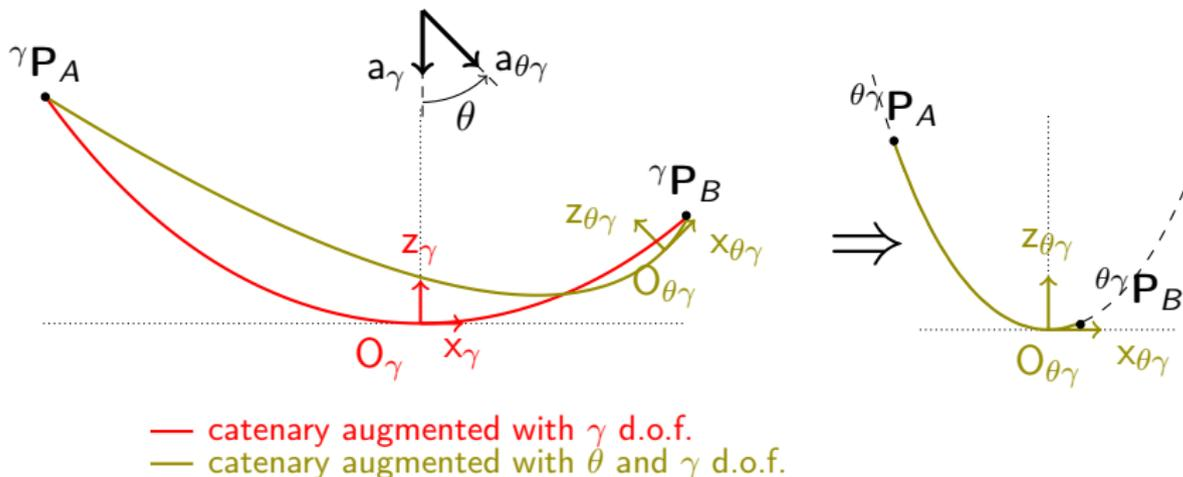
**Figure:**  $\gamma$  and  $\theta\gamma$ -augmented catenary of length  $L$  hanging between  ${}^w\mathbf{P}_A$  and  ${}^w\mathbf{P}_B$  in  $\mathcal{P}_\gamma$ .
